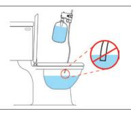
**Step 3:** Hold the Connector tightly with one hand and use the other hand to gently push the Connector lever (D) clockwise around the Connector.
